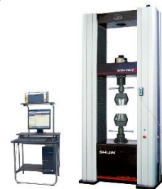
Fig. 5. Electronic Universal Testing Machine WDW-10E [1].
